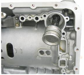
Make sure the servo rod and anchor pin is touching the band supports
