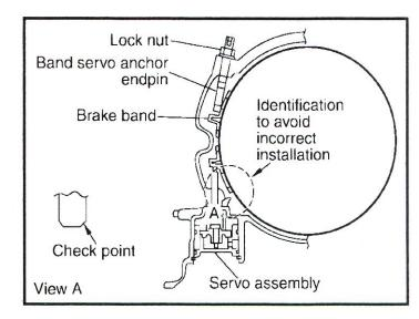
Tighten the anchor end pin to 50 in. lbs. for early models (2003-2005) and 44 in-lbs for late models (2006-up)
