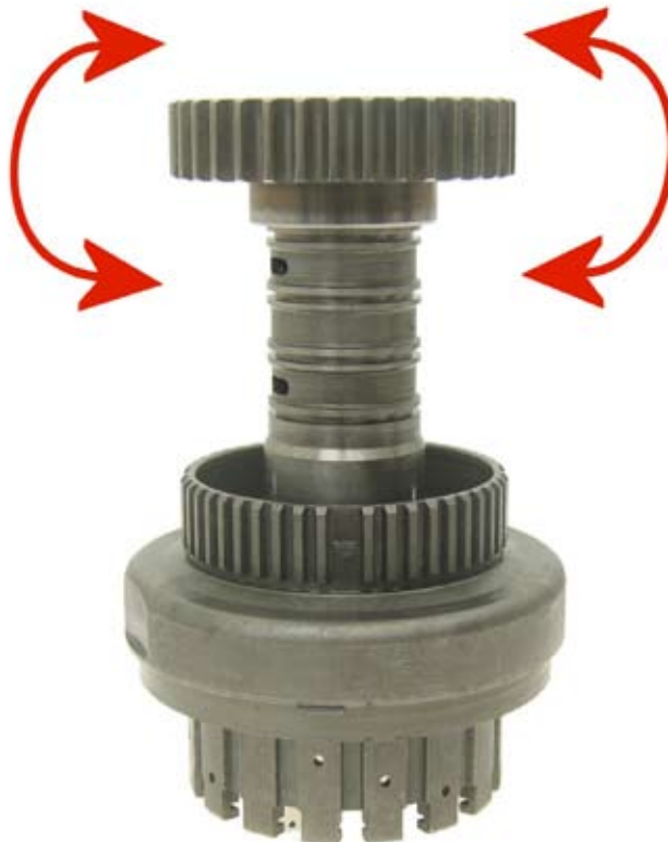
Figure 1 Checking Chain Sprocket Splines for Wear
