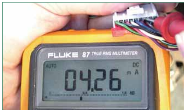
Figure 8 : Grounding DRAC harness connector terminal C13 to check DC current
