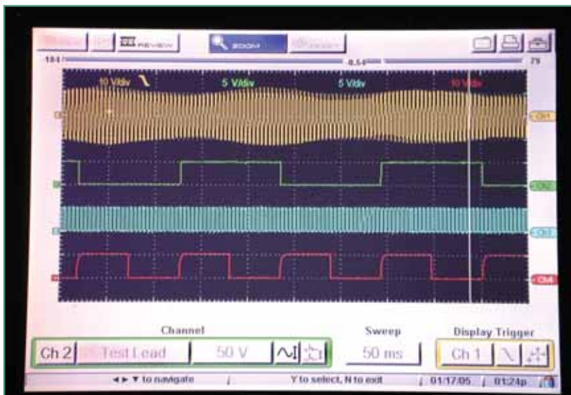
Figure 12: After zooming out, we can view more cycles of the Vehicle Speed and Speedometer signal waveforms
