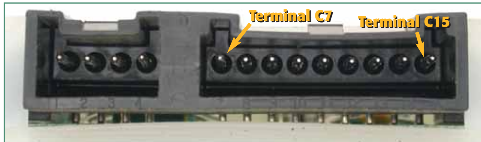
Figure 2: The 9 pin connector on the DRAC is where the power, ground, and main input/output signal connections are made
