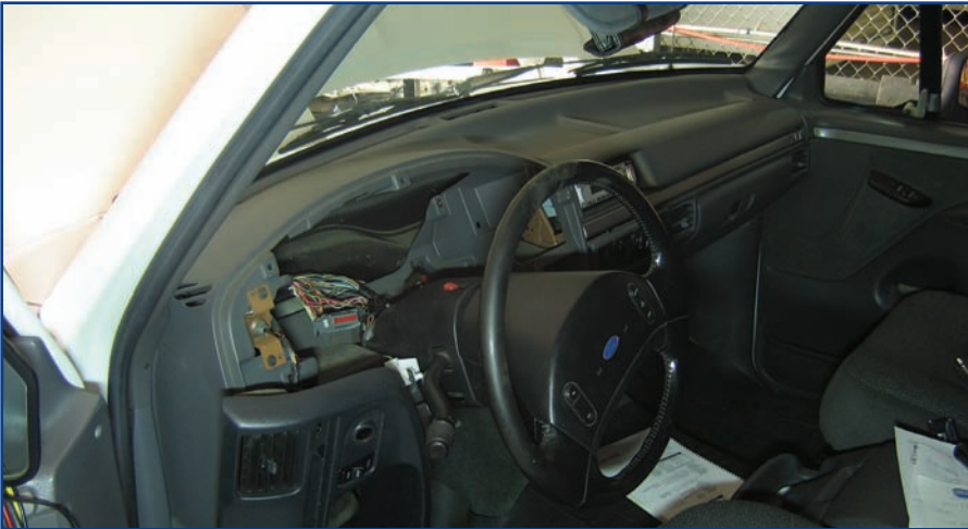
Figure 6: Once we narrowed down the problem, we removed the instrument cluster for further testing.
