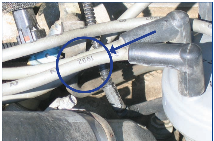
Figure 2: Original spark plug wires with 1992 year code were highly suspicious.
