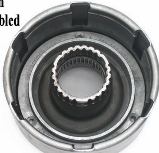
Figure 3: K2 clutch disassembled, inner seal hard and broken
