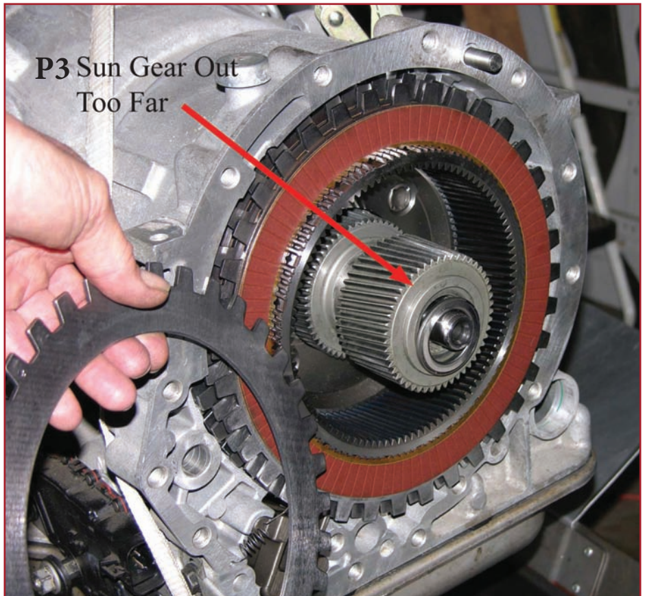
Figure 3: View of back end with things out of place.
