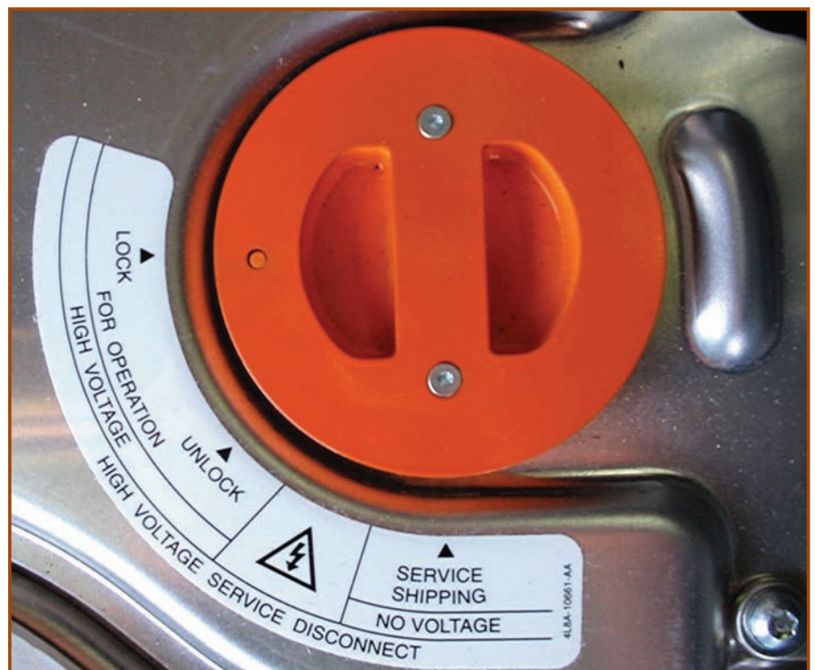
Figure 3: High voltage battery isolator
