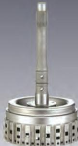
Manufactured exclusively by GFX, this ZF 5HP24 drum features our own Crocodile™ snap ring with teeth. This avoids cutting the drum, weakening the snap ring section, the major cause of failures.
