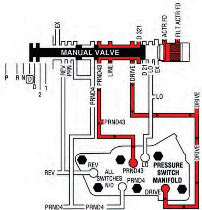
In the absence of the PCM to control solenoid operation, you can use the pressure manifold assembly to substitute the necessary ground signals to energize the solenoids in the proper combination to provide full manual control. Here's how:
