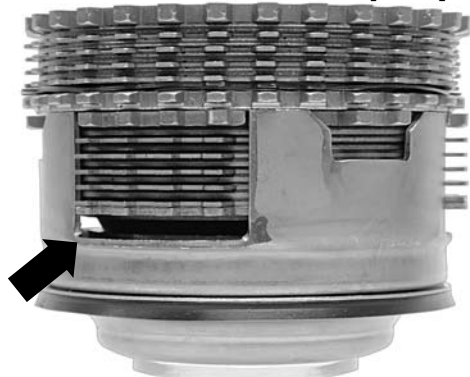
Clutch Stacked Properly
