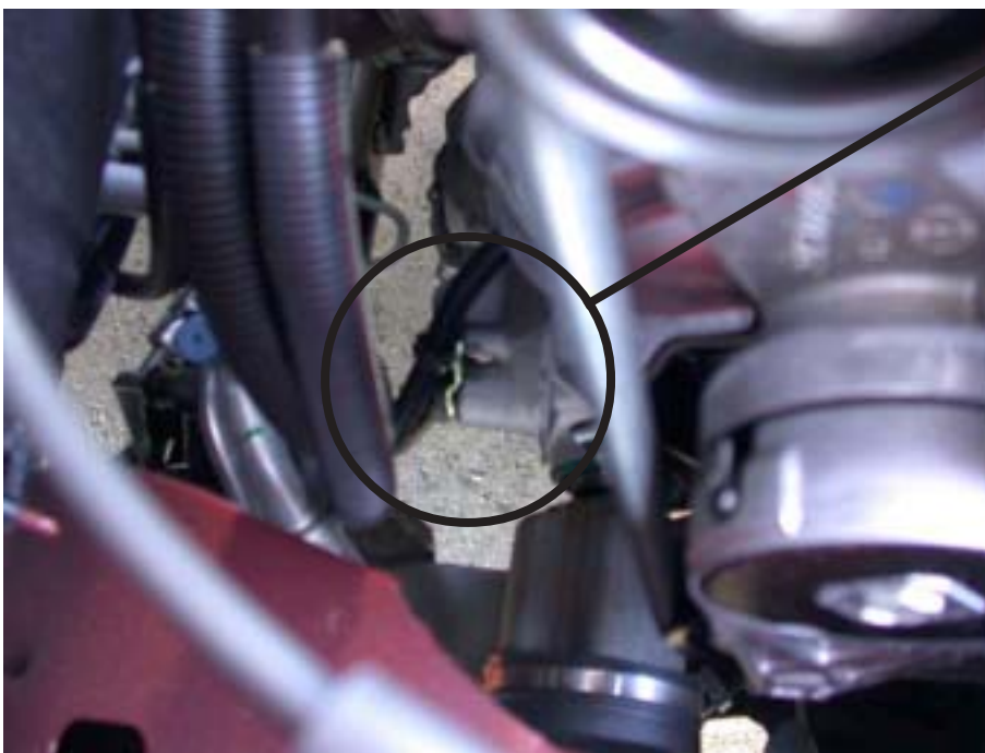
VSS harness the right hand (passenger side) axle shaft area.
