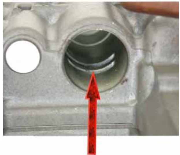
Line pressure from the regulator valve
