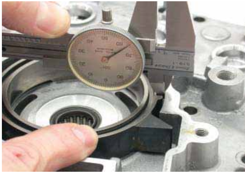
Measurement of the slide in the max position of its travel
