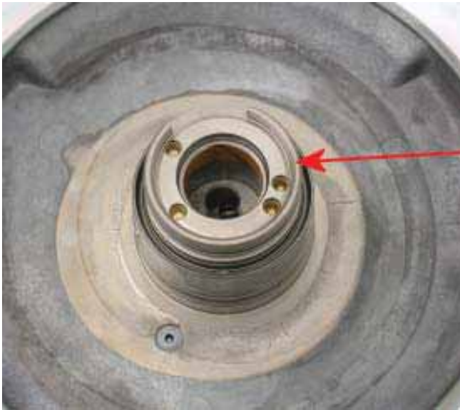
Hard Coat Anodized Aluminum Cover (Mazda Applications)
