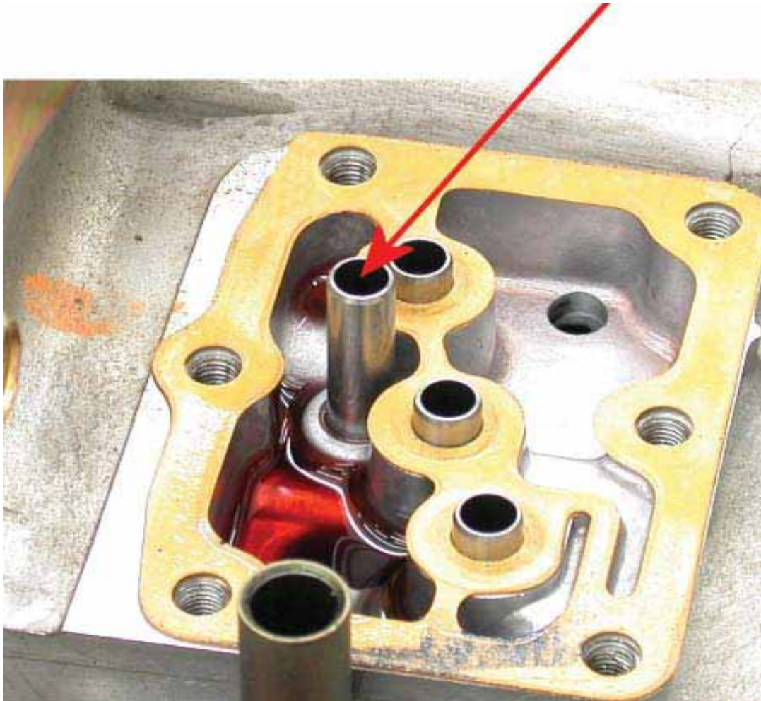
CPC Feed Pipes
