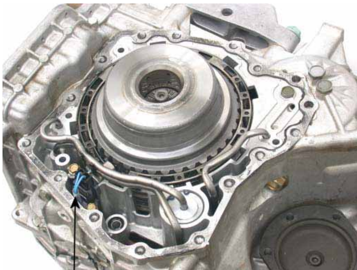
Input Speed Sensor (blue wires)
