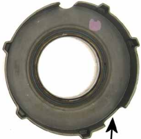
NOTCH FOR TURBINE SPEED SENSOR
