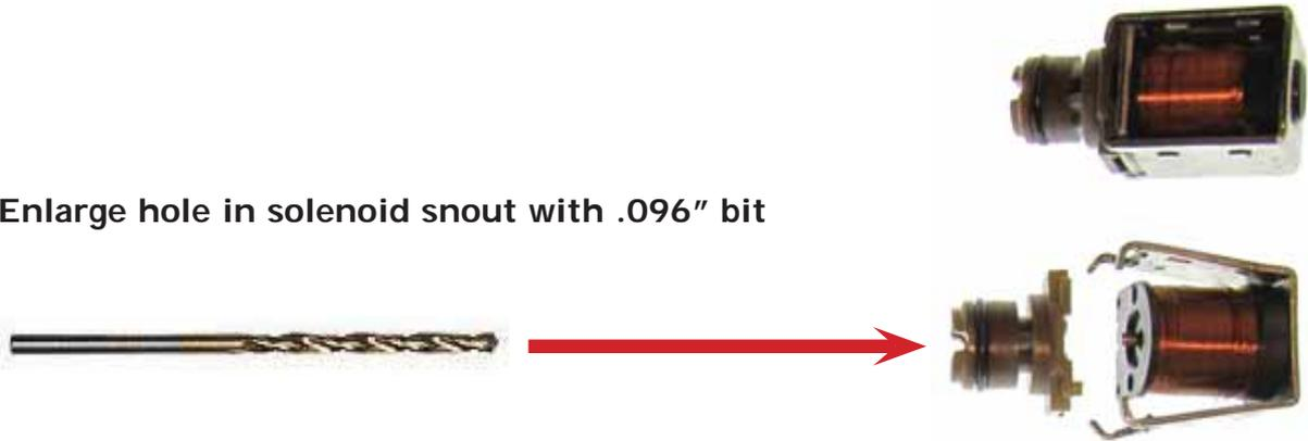
Install the modified solenoid snout and retainer clip into the "A" solenoid location. Leave internal harness plugged into the existing shift solenoid "A" so the ECM will not set a code and command both solenoids off (fail safe).
