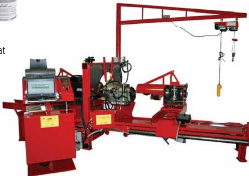
Dyno: Transmission Road Test Simulator
