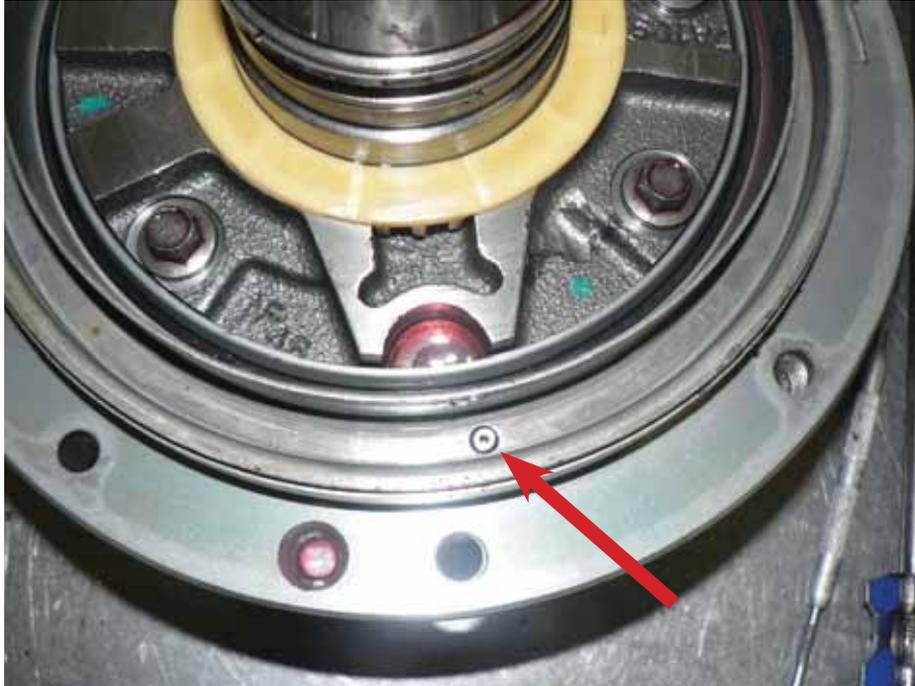
**Air Bleed Check Ball Capsule Falls Out Out When Piston Is Removed**
