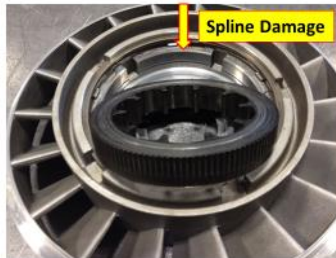
One Way Clutch outer splines damaged in the stator clutch pocket.
