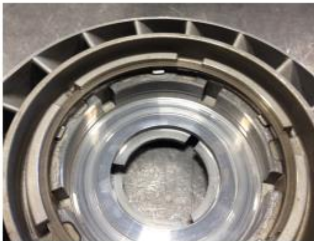
One Way Clutch outer splines damaged in the stator clutch pocket.
