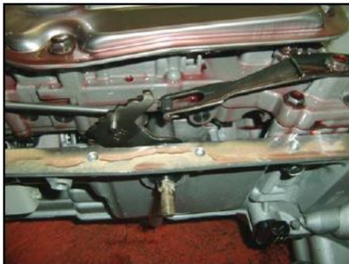
Figure 1. Detent Spring Detached from Manual Shift Lever (Transmission Oil Pan Removed for Clarity)
