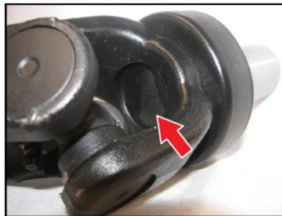
Figure 1. Area of Transmission Fluid Leak in Propeller Shaft (Driveshaft) Slip Yoke Plug
